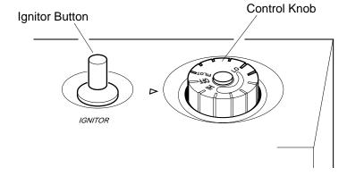
Figure 17 - Control Knob In The OFF Position
